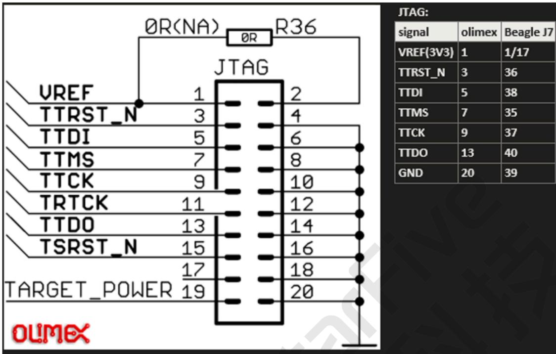
Figure 2-5 Connection Diagram
